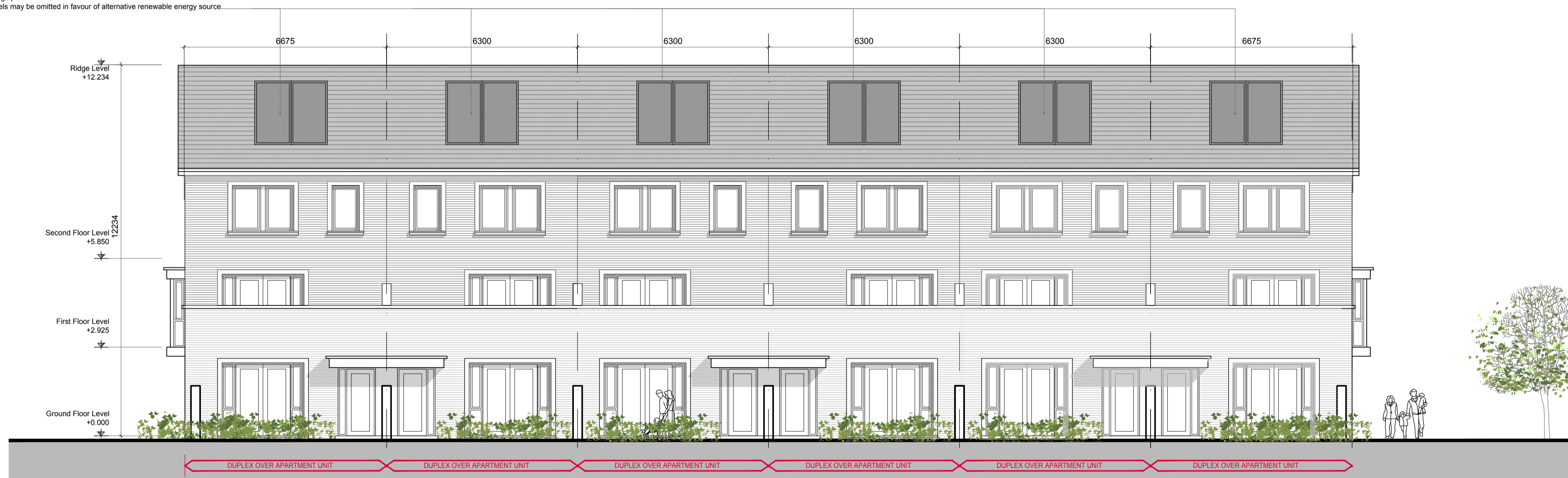
DUPLEX TYPE 2 - REAR ELEVATION DUPLEX TYPE 3B2 AT EITHER END
